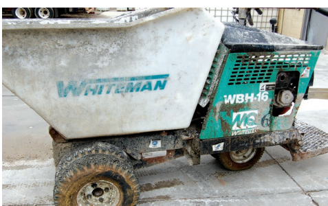
Power wheelbarrow before cleaning
