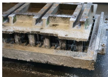
Bloc paving mould during cleaning
